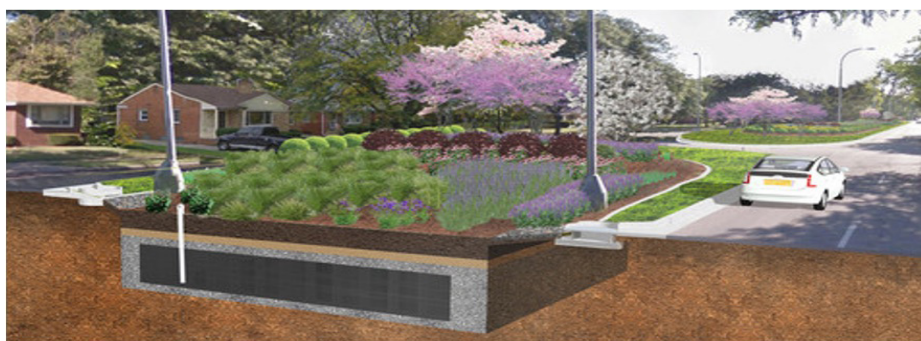
Figure 2.7, bottom: Computer rendering of a stormwater detention basin and garden for the median of Oakman Boulevard in Detroit. 75 Retrieved from DBusiness Magazine.
